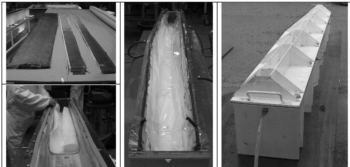
Fig. 1 Mould and manufacturing steps.
